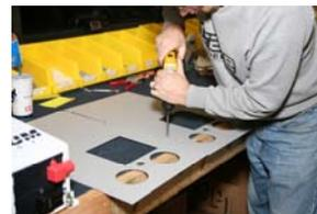
Pre-tapping inverter holes in door. Use four 10-32 (5mm) thread forming screws and four star washers to secure the inverter to the door
