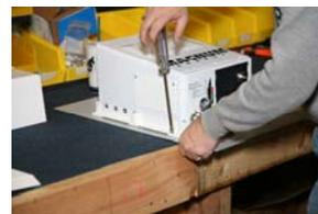
Installing the inverter to the door while still horizontal.
