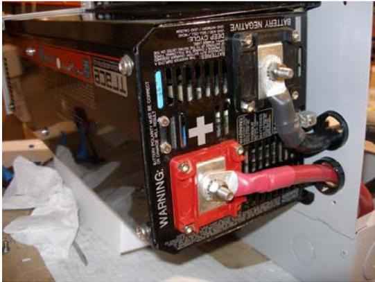
Connect up the DC inverter cables as shown to the left. Take special care to avoid hitting the ground terminal on the back of the DR/TR as it may cut through the inverter cable insulation. Make sure to install the snap in grommets prior to installing the inverter DC cables. Torque the DC terminals per the inverter specifications.
